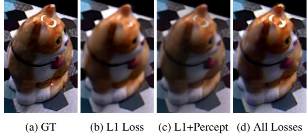
Figure 11: Effects of loss functions on neural-rendering. The specular highlights on the forehead of the Labcat is expressed weaker than it actually is when using L1 or perceptual loss, likely due to geometric and calibration errors. The highlight is best expressed when the neural rendering pipeline of Sec. 6 is trained with the combination of L1 , perceptual, and adversarial loss.
