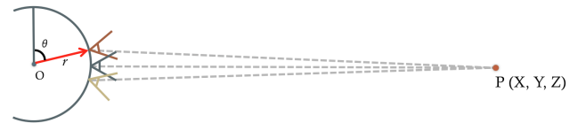
Figure 4: Top-down view of the simplified camera motion model, based on the arc radius r and orientation \theta .
