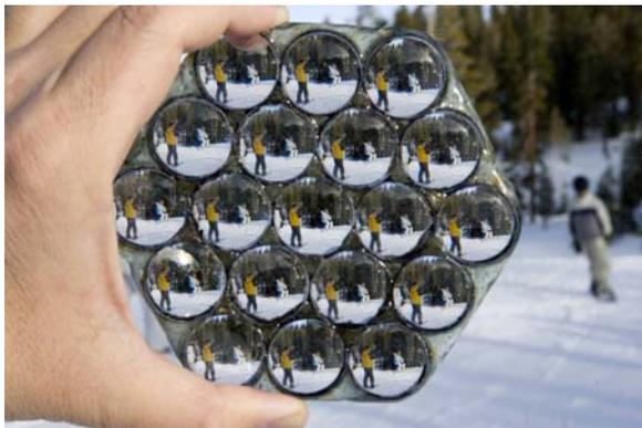
**Figure 4:** Our optical device consisting of lens-prism pairs.
