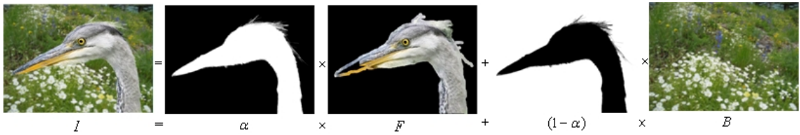
Figure 1.3: In the image matting problem the observed image I is modelled as a convex combination of a foreground image F and background image B . The interpolation coefficient \alpha is called the matte .
