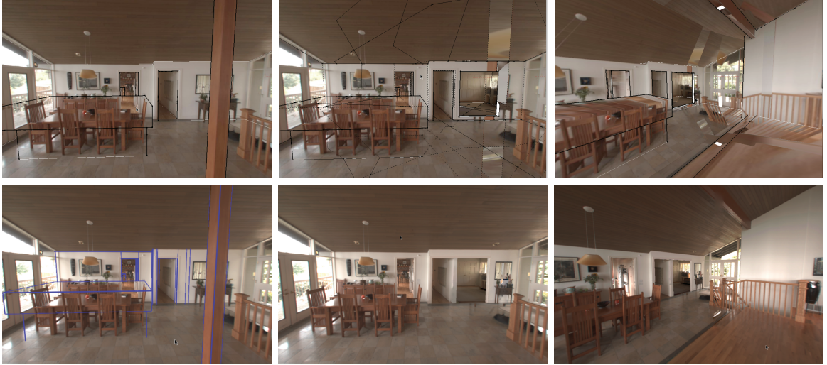
Figure 4.2: Comparison of Google Sketchup’s Photomatch using geometry exported from our system. Top row: Google Sketchup, Bottom row: My System. In the center images, the column was removed and a passage opened into a study. Note how Sketchup breaks up polygons due to original occlusions in the image projections. This makes remodeling almost impossible. Also note poor textures in revealed and new surfaces. Right: the same edit viewed from a different viewpoint. My view dependent texture automatically utilizes texture relevant to the new viewpoint.
