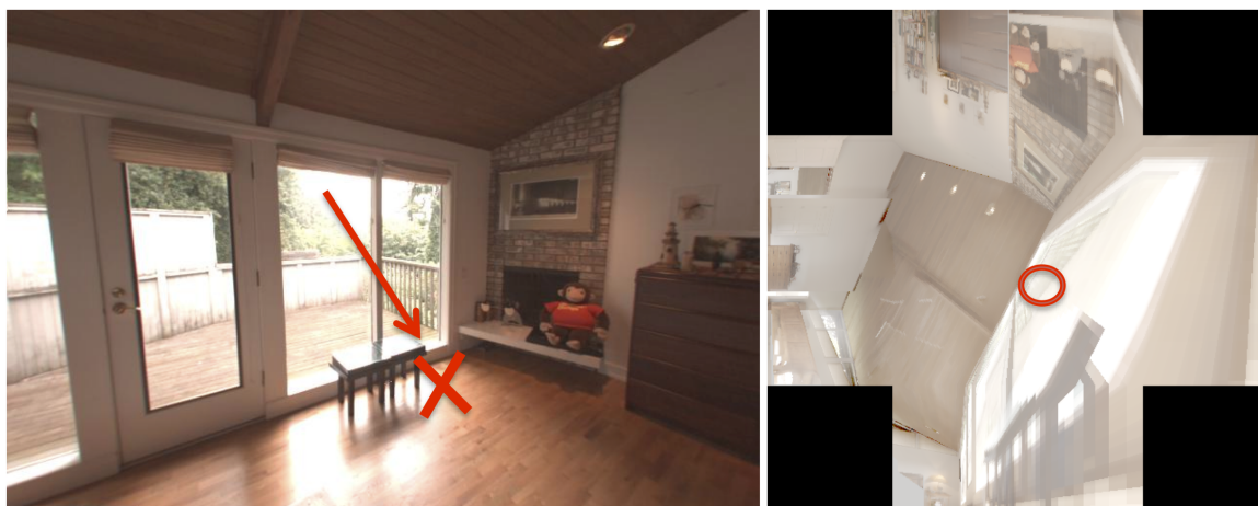
Figure 5.1: Left: A point on the floor receiving light from the window. The point on the floor is marked with an X , and a ray of light from the exterior is indicated with an arrow. Right: A rendered image from the viewpoint of the point on the floor. This image is rendered using a global texture map (the VITA) to represent the light coming in from the window. Since this texture is generated from a different viewpoint from the point on the floor, the source of the ray of light indicated by a circle does not have the same intensity as the actual ray of sunlight. Any rendering from this viewpoint using a VITA will mis-represent the light intensity of the scene. In this case, the ray of sunlight is not captured from any viewpoint and the intensity error is so great that it can not be reliably used for any subsequent calculations.
