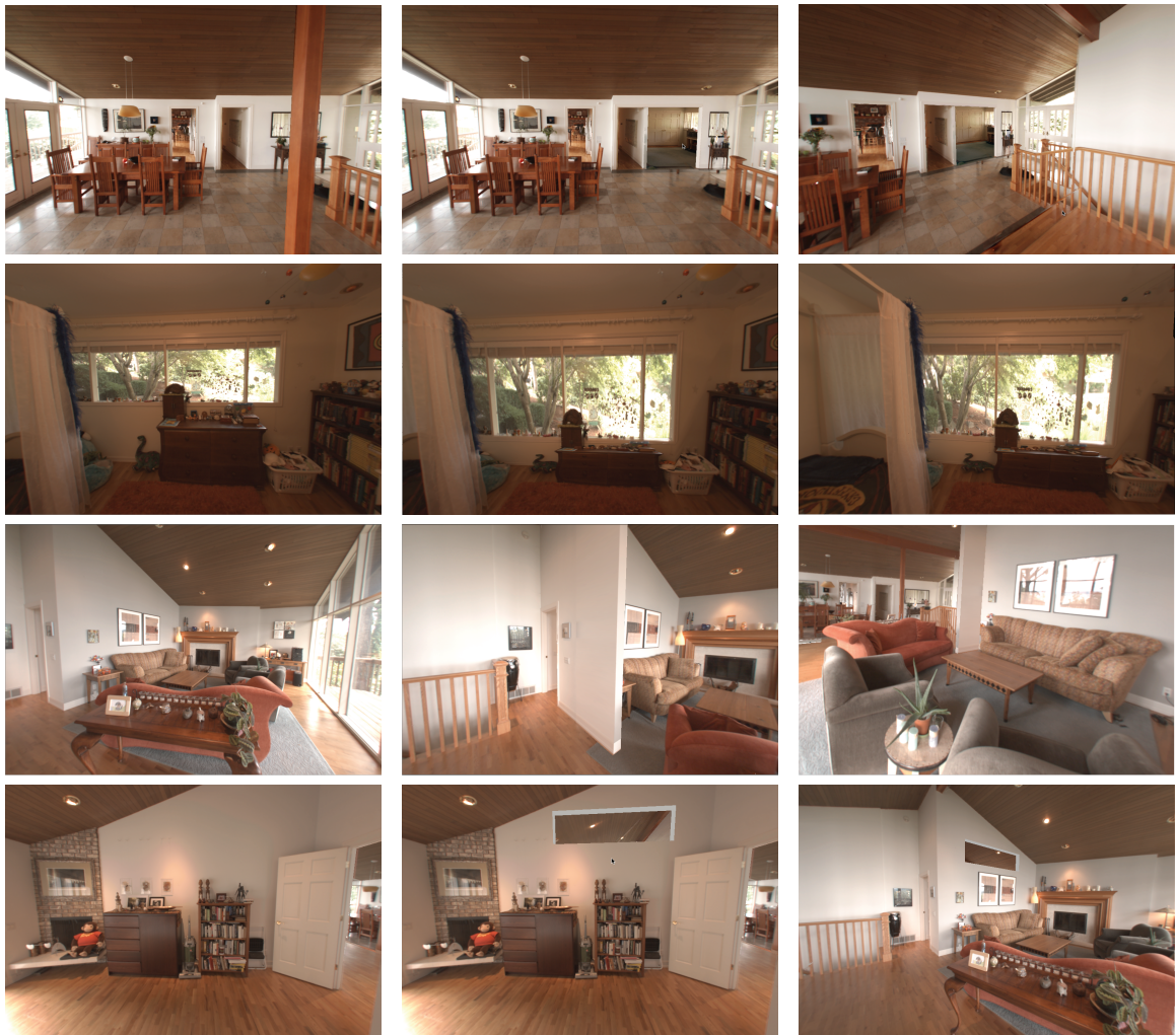
Figure 4.7: Three remodeling results. First column: original viewpoint. Second column: remodeled geometry. Third column: same remodel from different viewpoint. First row: opening a wall to connect two rooms. Second row: expanding a window vertically. Third row: adding a wall segment. Fourth row: creating a cutout.
