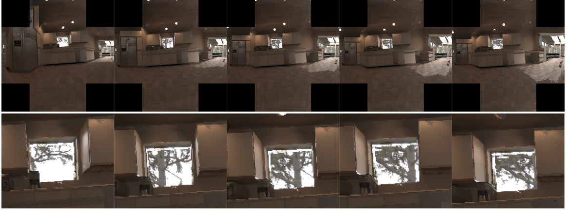
Figure 5.8: Top row: A hemicube view changing position from left to right. Bottom row: The kitchen window regions that utilizes an LRI lighting function is enlarged to enhance the view. The direct natural light function that computes L(x \rightarrow \Theta) utilizes an LRI panorama. In this example we can see that the light computed by the LRI changes as hemicube position changes. The kitchen window is a natural light, and as the hemicube viewpoint changes, so too does the incoming light from the window. The tree located outside the window appears to move from left to right as it comes in and out of the field of view.
