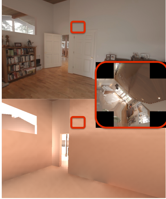
Figure 5.5: Top: original image. Bottom: Irradiance calculated by hemicube integration at every pixel using a VITA texture mapped rendering. The rendered intermediate image used for the hemicube calculation is shown for the point marked by the red square.
