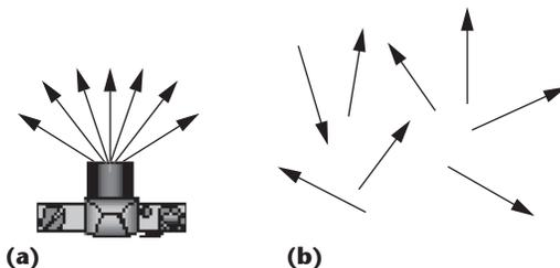
1 Set of rays corresponding to (a) a perspective image and (b) a multiperspective image.
