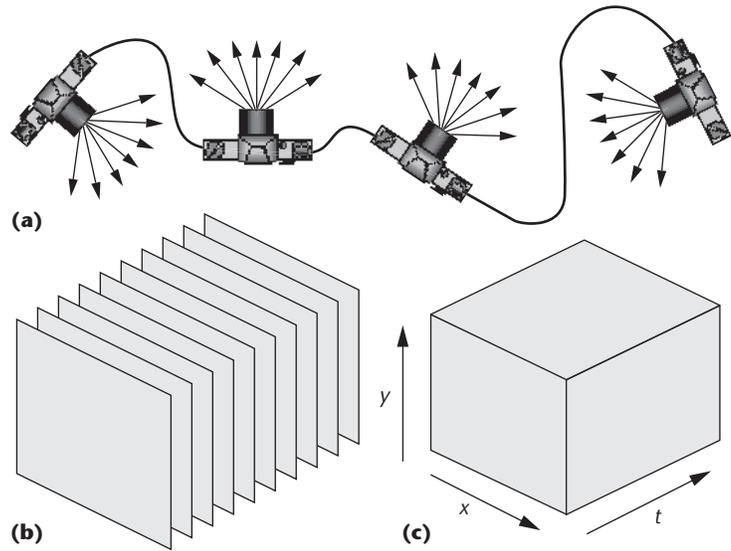
**2** (a) A camera moves along a path and captures light rays. (b) Stacking the images one on top of another yields (c) an  $x$ - $y$ - $t$  video cube. Each slice of the video cube produces a path image and represents a subset of the captured light rays (shown figuratively in red).
