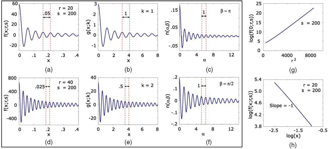
Fig. 2. Left:  $f$ ,  $g$ , and  $n$  functions for two different values of frequency cut-off  $r$ . As  $r$  increases,  $f$  becomes more and more oscillatory with period  $\frac{1}{r}$ . The period of  $n$  however does not change. Right: (g) shows that the amplitude of  $f$  (at  $x = 0$ ) increases exponentially with  $r^2$ . The log-log plot (h) of amplitude of  $f$  versus  $x$  is a straight line with slope  $-1$ , showing that the filter falls off as  $\frac{1}{x}$ .
