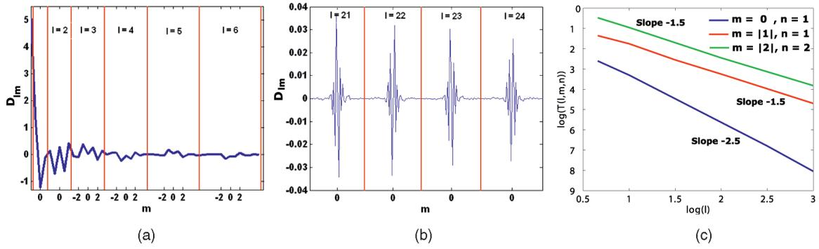
Fig. 8. (a) and (b)  $D_{lm}$  plots for low and high frequencies. Note that  $D_{lm}$  coefficients are small for  $|m| > 2$  and, hence, can be safely neglected. (c)  $T_{lmm}$  plot.  $T_{lmm}$  falls off rapidly as  $l^{-3/2}$  or  $l^{-5/2}$  for  $l \geq 2$ .
