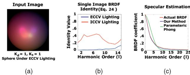
Fig. 9. (a) Synthetic sphere image with both diffuse ( $K_d$  set to 1) and specular (taken from measurements of a real material) components. (b) Image consistency checks (24) can distinguish small inconsistencies between illumination and image ("ECCV" versus "ICCV" lighting). (c) For estimation of  $A_l$ , our approach gives accurate results, outperforming a parametric estimation technique.
