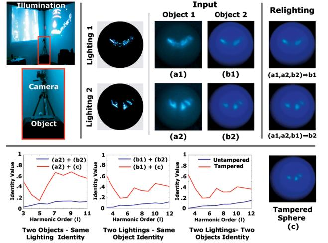
Fig. 11. Top left: Experimental setup. Top middle: Two lightings (shown only for reference) and images of two glossy (diffuse plus specular) spheres in that lighting. Top right: We can accurately render (b1), given (a1, a2, b2), and render (b2), given (a1, a2, b1). Bottom: We tamper (b2) to generate (c) by squashing the specular highlights slightly in photoshop. Although plausible to the naked eye, all three identities in Section 6 clearly indicate the tampering (red graphs).
