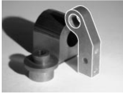
Figure 17: The final pose obtained using the solution in Figure 16 as the initial solution to a non-linear least squares pose estimation procedure. Note that the gap between the object and its features is now gone.
