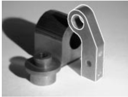
Figure 16: The pose computed from six point correspondences and one ellipse-circle correspondence using the generalized methodology. Note the gap between the object and the projected model at the very top of the object.
