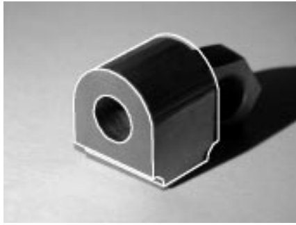
Figure 19: The pose computed from an ellipse-circle correspondence using the algorithm described in Section 5.6.
