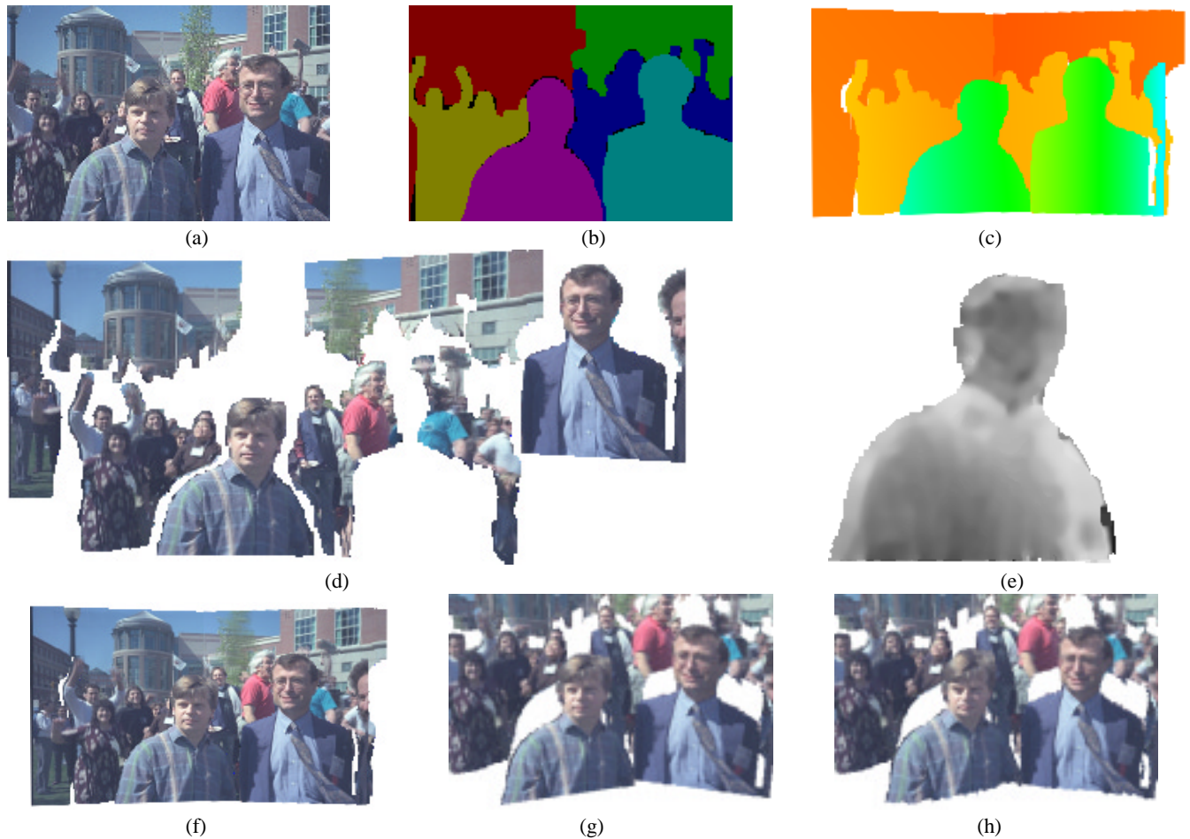
Figure 4 Results of sprite extraction from image sequence: (a) third of five images; (b) initial segmentation into six layers; (c) recovered depth map; (d) the five layer sprites; (e) residual depth image for fifth layer; (f) re-synthesized third image (note extended field of view); (g) novel view without residual depth; (h) novel view with residual depth (note the "rounding" of the people).
