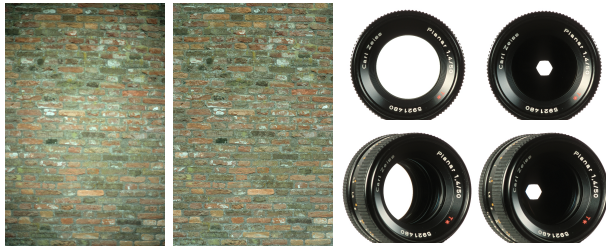
Figure 3 Left: image of a wall at f/1.4 . Middle: same wall at f/5.6 , showing that optical vignetting decreases with aperture size. Right: the shape of the entrance pupil varies with both the aperture ( x axis) and the angle of incidence ( y axis). The white openings correspond to the clear aperture for light that reaches the image plane. © Paul van Walree.
