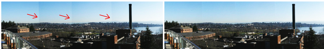
Figure 1 On the left, a panoramic sequence of images showing vignetting artifacts. Note the change in brightness at the edge of each image. Although the effect is visually subtle, this brightness change corresponds to a 20% drop in image intensity from the center to the corner of each image. On the right, the same sequence after vignetting is removed.
