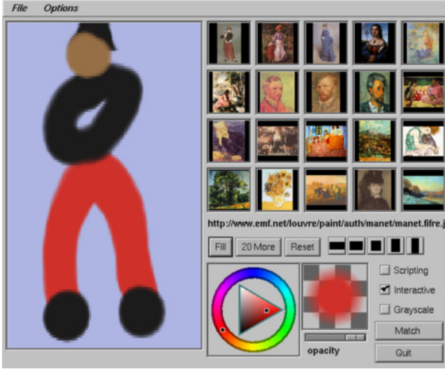
Figure 1: The image querying application. The user paints a query in the large rectangular window, and the 20 highest-ranked targets appear in the small windows on the right. To avoid copyright infringements, the database for this example contains only 96 images (all created by artists who have been dead more than 75 years). Because the database is so limited, only the intended target (in the upper-left small window) appears to match the query very closely.
