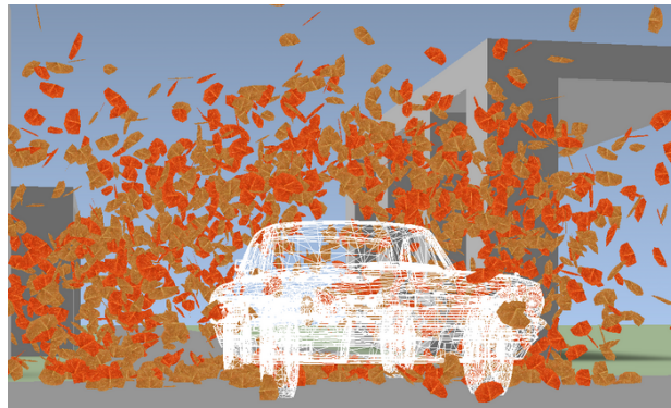
Figure 1: An interactive fluid simulation of a car driving through 4000 leaves runs at 24 frames/second on a 256×64×128 grid. (Car model courtesy of Digimation.)
