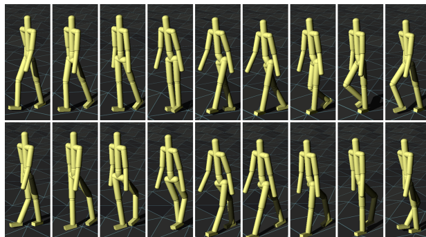
Figure 4: Applying the unaltered forward controller to two different bipeds: one with its left knee frozen (top), and one with inverted knees (bottom).
