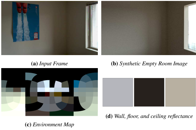
Figure 4: Recovered distant illumination parameters. (a) is an input image from the capture sequence. (b) shows a rerendered version with our distant lighting model. (c) shows a (\theta, \phi) parameterization of the recovered cubemap; note that the central region corresponds to the directions out the window. While this approximation does not appear representative of the actual appearance out the window and only imprecisely matches shadow boundaries, it captures most of the illumination effects that affect the indoor scene. (d) shows the recovered wall, floor, and ceiling reflectances. In the actual scene, the wall and ceiling have identical properties; the solved reflectances are very similar even though we did not constrain them to be the same in our system.
