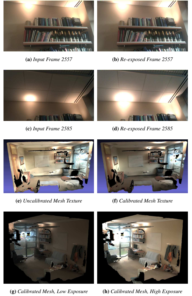
Figure 2: Comparison of office mesh, before and after radiometric calibration. (a) and (c) are two of the original input frames showing a similar area of the scene; note that (c) is significantly darker in appearance than (a) due to autoexposing for the lights. (b) and (d) are derived from (a) and (c), respectively, but rescaled to have the same exposure level. (e) shows a naive texturing of the scene geometry without any exposure correction; there are many noticeable artifacts on the wall. (f) shows the texturing after radiometric calibration (linearly tonemapped and clipped). The artifacts on the wall have been completely smoothed. (g) and (h) show another view of the mesh with calibrated texture at differing exposure values; notice how the lights are all brought within range.
