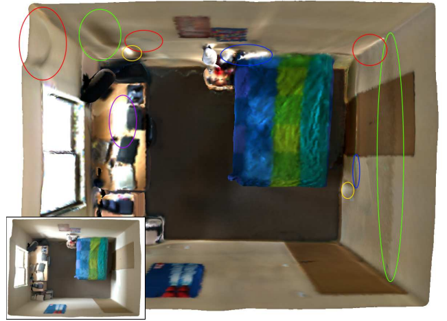
Figure 11: We compute a “reflectance mesh” by taking the radiances from the input mesh (inset) and the solved lighting, and compute a per-vertex reflectance as radiance divided by incident light. We expect that the walls will have a uniform reflectance, but some artifacts are visible. The red circles show regions where the inaccurate wall geometry results in inaccurate normals. The blue circles show regions where the inaccurate scene geometry results in incorrectly projected scene radiance. The yellow circles show regions where the inaccurate scene geometry results in incorrect occlusion boundaries. The green circles show artifacts from the low resolution of the lighting. The large white spot on the desk (circled in purple) is due to the specularity of the desk; the radiance given by the input mesh is an overestimate of the diffuse appearance of the desk, and thus the computed reflectance is also too high. Although not an issue in this case, this specularity can also cause an overestimate in the the incident indirect illumination on other points in the scene.
