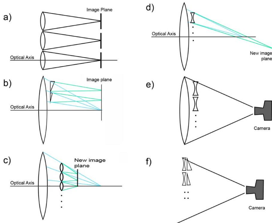
Figure 5.3: Six designs of light field cameras. (a) Integral photography. (b) One lens and multiple prisms. (c) Main lens and a lens array - used in integral photography. (d) Main lens and an array of negative lenses. (e) Same as 5, only implemented as *external* for the camera. (f) Example of external design of negative lenses and prisms that has no analog as internal.
