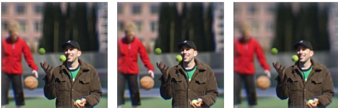
(c) Synthetic aperture results with varying depth of field. (Left image demonstrates sparse sampling.)
