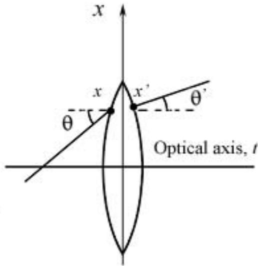
Figure 5.2: Light field transformation at the plane of a lens.
