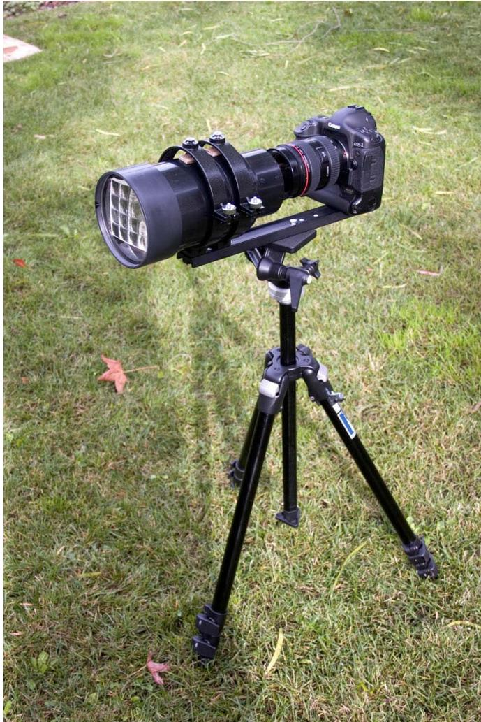
Figure 5.6: Our sparse light field camera prototype, with 2 positive lenses and an array of 20 negative lenses in front of a conventional camera.
