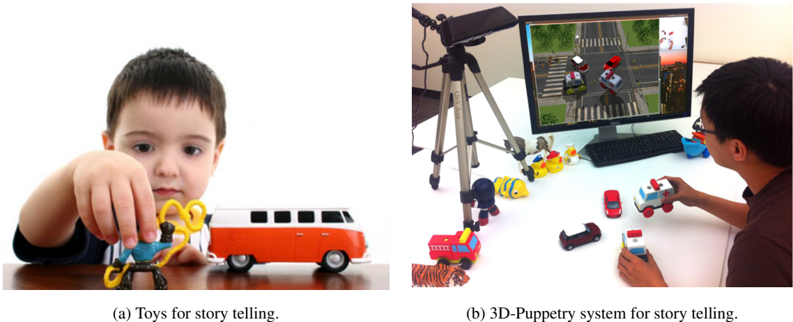
Figure 4.1: Natural and intuitive interfaces for story telling. (a) Toys and puppets are the traditional ways of natural story telling. (b) The 3D-Puppetry system tracks the moving physical objects using a Kinect® camera and renders their tracked virtual replicas on the screen in realtime to create an animated story.
