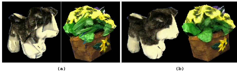
Fig. 6. (a) The result of combining three views by repeatedly rendering the view-based meshes from the viewpoint of the virtual camera. (b) Using the weights and soft z-buffering produces a much better result.
