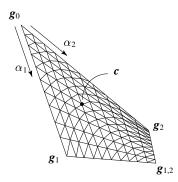
Figure 2 Bilinear surface described by the Neugebauer halftone model.
