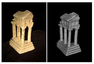
Figure 1. Reconstruction (*right*) from the *templeFull* dataset and an input image (*left*) for comparison. Despite the simplicity of the proposed algorithm, it is able to estimate the object's shape to sub-millimeter accuracy.
