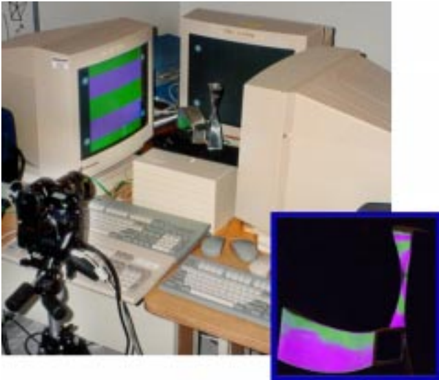
Figure 3 A photograph of the experimental setup used to capture environment mattes. The camera in the foreground photographs objects surrounded by structured light patterns displayed on the computer monitors. The image is processed to extract only the area covered by the backdrop pattern, resulting in an image as shown in the inset.
