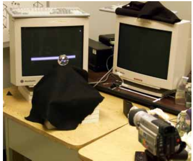
Figure 4 A photograph of our experimental setup. In this instance an accurate environment matte is being acquired.
