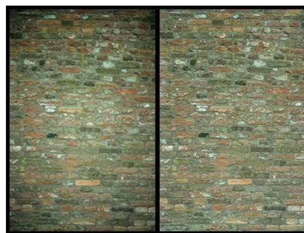
Optical Vignetting: occlusion after aperture
