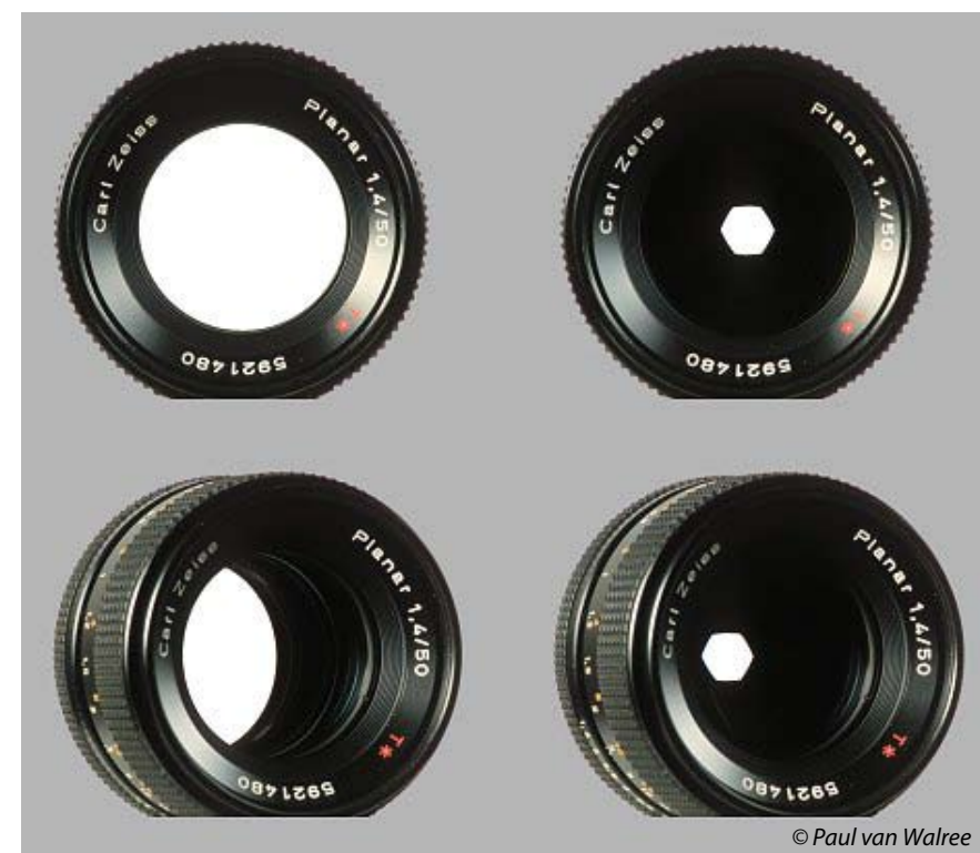
Optical Vignetting: occlusion after aperture
