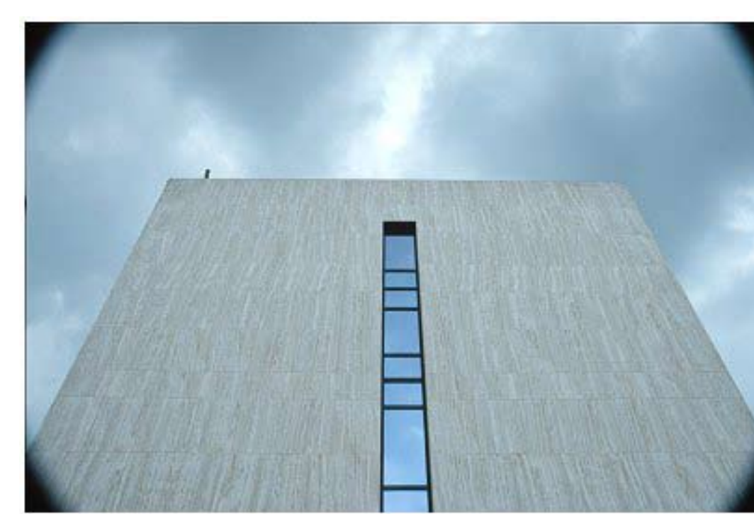
Mechanical Vignetting: occlusion before aperture
