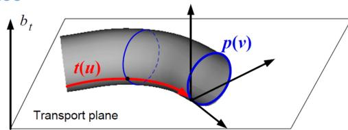
Given a transport curve  $t(u)$  with unit speed parameterization and a profile curve  $p(v)$ , the rotation applied to the profile curve at each point  $t(u)$  is defined as
