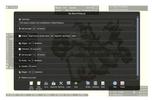
Figure 1: A screenshot of the cookbook editor for a GUI recipe. The visual blocks that make up the recipe take up the main section of the window. Buttons for saving, loading, sharing, and other options are along the bottom.
