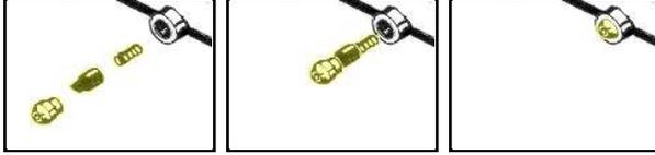
Figure 12: Multiple parts in a stack can interlock. Here all three highlighted parts interlock with the hole. Our semi-automatic depth assignment algorithm uses constraint propagation to automatically choose depth values for all of these parts so that they are properly layered between the front and back fragments of the hole.
