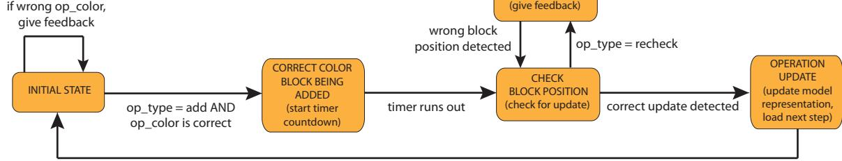
Figure 5: The Update Detector is implemented as a finite state machine with user input and tracked data as input to update the model. In Authoring mode, it detects an update and applies it unless a recheck is requested by the user. In Guidance mode, it detects and performs the update and displays feedback to the user if there is a mistake.
