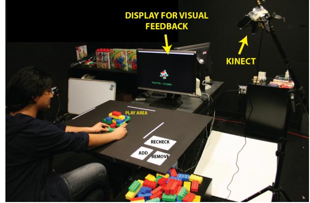
Figure 1: System setup. The user builds the model in the *Play area* and uses the *Add/Remove/Recheck boxes* to interact with the system. The Kinect® looks down from the right and passes the captured video/depth stream to our system to track the model and infer the assembly process in realtime. Visual feedback is shown on the display in front of the user.
